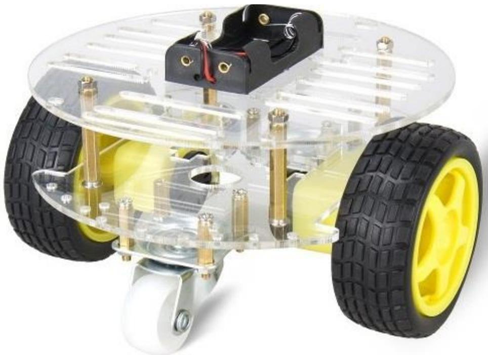
Gambar 1. Kit Round Chasis Mobile Robot [2]
